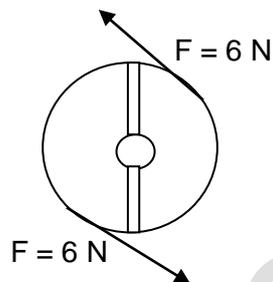
Assuming that the steering wheel has a diameter of 400 mm, determine the moment associated with these forces.
