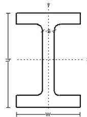
Properties of some British Column and Beams according BS 4.
